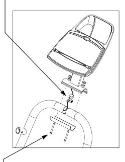
(D), two washers (B), and two locknuts (C). Finger tighten.
